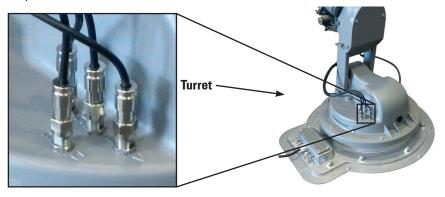
4 Remove the bolt holding the cable harness to the unit, and detach the cable harness from the lift arm.
