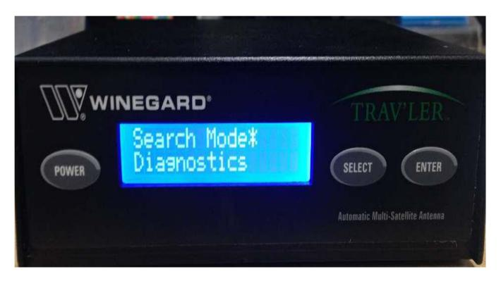
4 - On the IDU box, press select once. It will move the asterisk next to Diagnostics. Then press ENTER once the asterisk is next to Diagnostics
