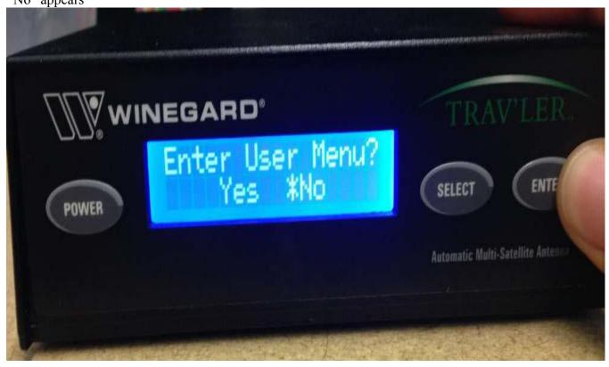
3 – On the IDU box press select to move the asterisk over to Yes, then press ENTER on the IDU box.
