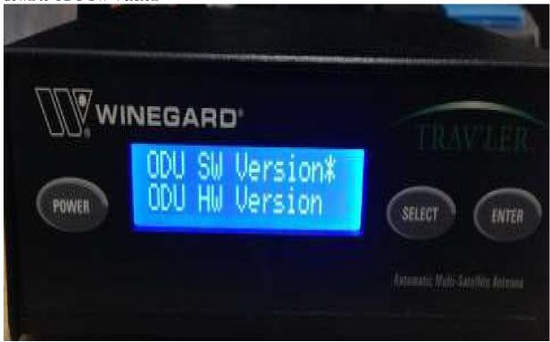
Press ENTER to get the ODU Software version of the Trav'Ler. After you can see the ODU software version, press ENTER to get back to the Menu selections.
